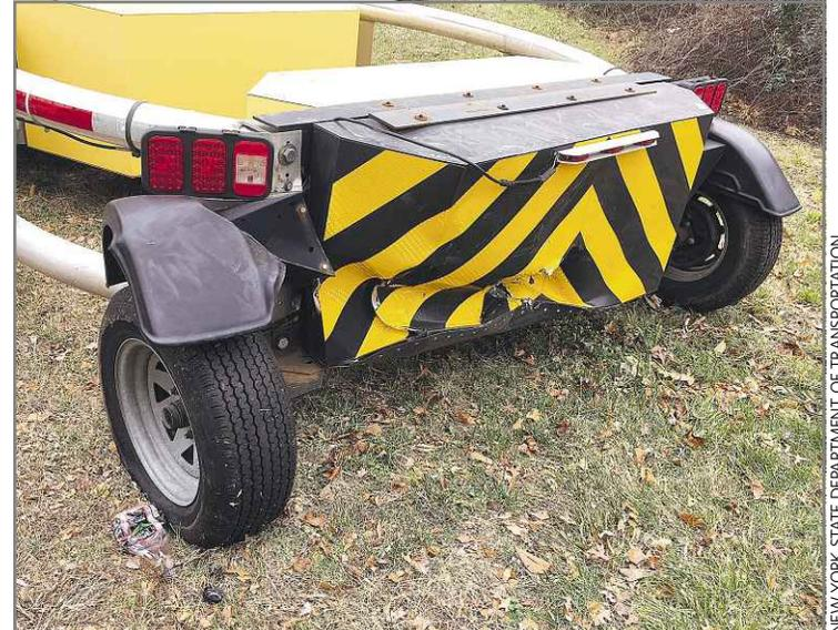
A Department of Transportation impact attenuator shows damage after it was hit by a vehicle Nov. 30 on the Meadowbrook State Parkway.
