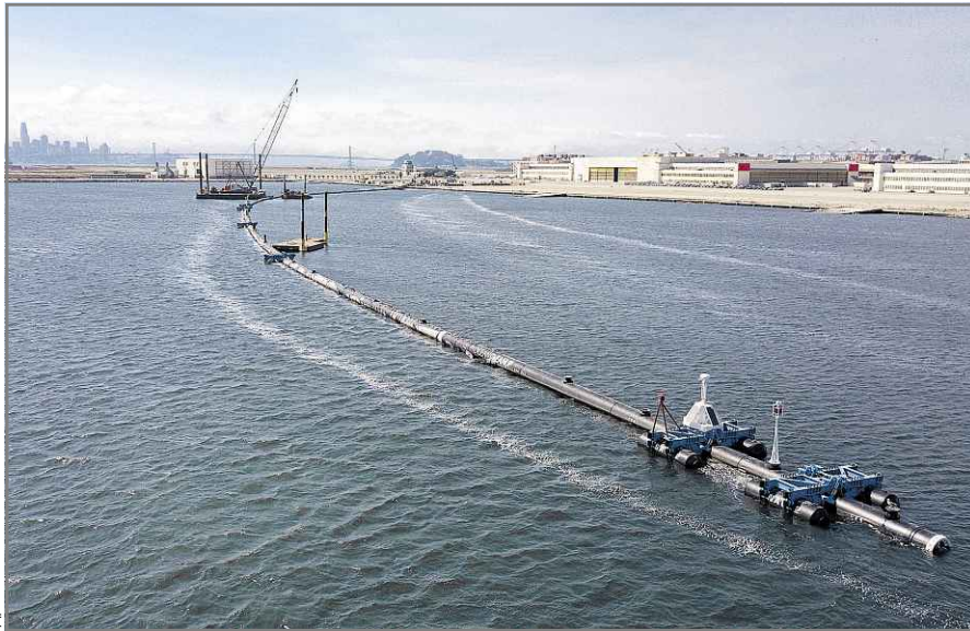
The 2,000-foot trash collection device by The Ocean Cleanup will be used to trap some 1.8 trillion pieces of plastic from the Great Pacific Garbage Patch.
